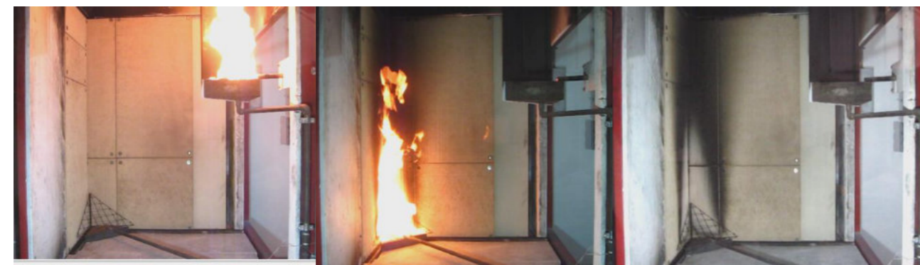
Figure 1 Recordings before, during and after SBI-Test DIN EN 13823 on econitWood Panels
